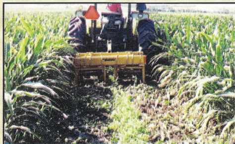
Two-Row Seed Corn Male Row Eliminator Chopper.
