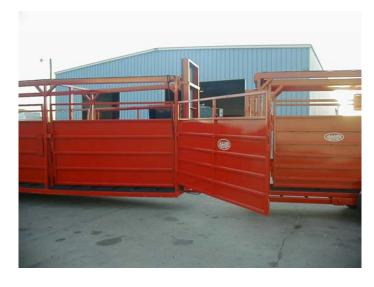
2-8' Panels fold out (1 per side) to make an additional 8' Alleyway
