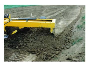
Standard adjustable-tilt axle allows precise depth control on either side of the scraper
