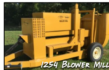
PTO 1254 ROLLER MILL W/INLET AUGER AND 18' DISCHARGE
