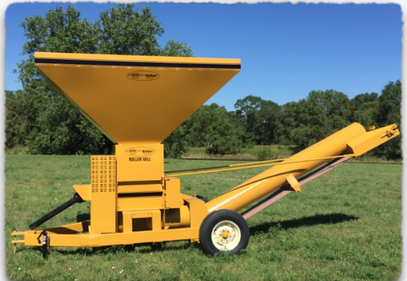
1227 W/80 BUSHEL HOPPER, 13' BELT DISCHARGE
