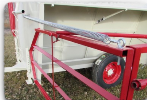
LOW EFFORT PATENT PENDING SPRING LIFT ASSIST PANELS
