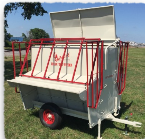
EASY FILL LID WITH PANELS UP OR DOWN
