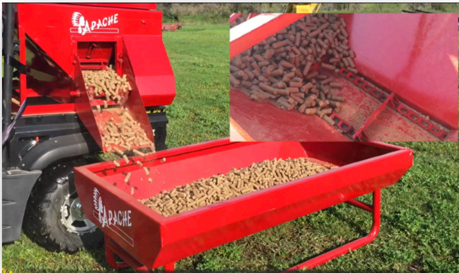
EXPOSED CONVEYER AND PADDLES ALLOW FLEXIBILITY OF RATIONS FED AND PREVENTS BRIDGING OF MATERIALS.
