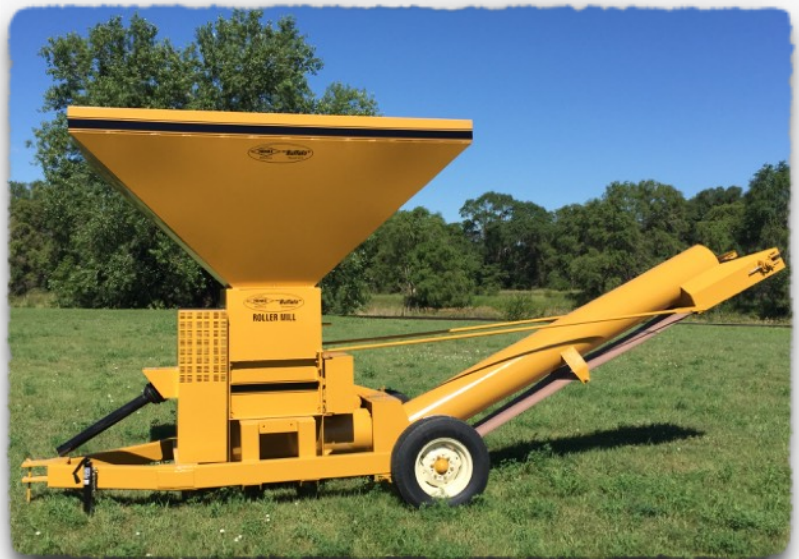
1227 W/80 BUSHEL HOPPER, 13' DISCHARGE BELT
